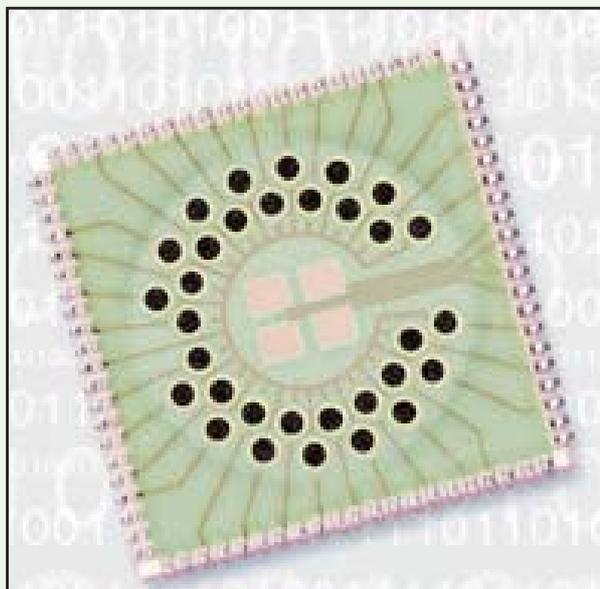
A Cyranose chip with 32 proprietary composite polymer sensors. From: Skelley, (2000) with acknowledgment to Cyrano Sciences, USA.
